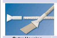
STATOMIX™ MCH static mixers were developed for the MIXPAC® 200 and MIXPAC® 400 cartridge system. The unique element design achieves proper mixing with minimal resistance, which is highly beneficial for manually powered dispensing. The MCH Cartridge static mixer has an industry standard connection of 16,7mm which allows it to be used with other cartridge systems
