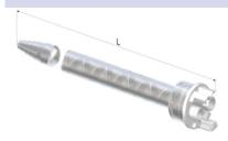
The STATOMIX™ MFH and MFHX mixers were developed for the MIXPAC® F200ml and MIXPAC® F400ml cartridge systems. The F system mixers feature a unique, state-of-the-art interface design between the static mixer and the cartridge. This interface features separated outlets which eliminates the possibility of cross contamination and curing at the mixer tip.
