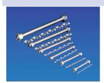
The AE Series stainless steel tube mixers are fitted with removable elements and are designed for use with 2-component reactive silicone elastomers, silicone foams and resin systems with fillers where cleaning is not possible by burning out the mixer content.
